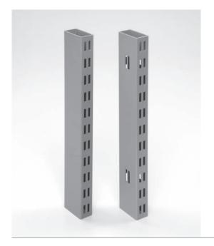
RECTANGULAR TUBE 60/30 PITCH 35 Product 60x30x2 mm double slottet two-sided or two-sided with side slots every Description 245 mm. Slot pattern 19 x 5 mm. Pitch 35 mm. **RAW** steel Material Sizes Length Perforation Article 60x30x2 6000 **DS 2**-s 13.6302.00 60x30x2 6000 DS 2-s + SS13.6304.00
