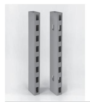
**RECTANGULAR TUBE 60/30** Product 60x30x2 mm wide single slotted, two-sided or two-sided with side slots Description every 250 mm. Pitch 50 mm. Slot pattern 28 x 14 mm. **RAW** steel Material Sizes Length Perforation Article 60x30x2 6000 SS 2-s 10.6320.00 60x30x2 6000 SS 2-s + SS10.6321.00
