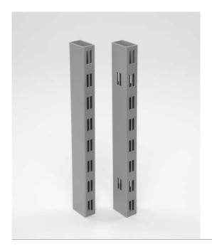
Product Description 50x30x2 mm double slotted, two-sided or two-sided with side slots every 250 mm. Slot pattern 28 x 5.2 mm. Pitch 50 mm.
