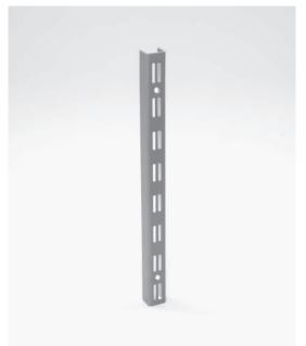
WALL RAIL DS HEAVY DUTY Product Heavy duty vertical rail for wall-mount double slotted. Description Slot pattern 28 x 5 mm. Pitch 50 mm. Sold per unit. RAW steel Material Depth Perforation Width Length Article 30 23.5 2400 DS 16.3003.00 Ral 9001 steel Material 2400 DS 16.3003.01 30 23.5 Ral 9006 steel Material 30 23.5 2400 DS 16.3003.02
