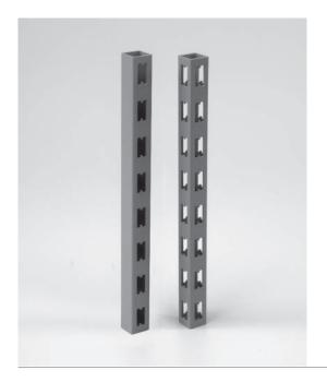
SQUARE TUBE 30/30 H Product 30x30x2.5 mm with H-shaped slots, two-sided or four-sided. Description Slot pattern 28 x 14.5 mm. Pitch 50 mm. **RAW** steel Material Sizes Length Perforation Article 30x30x2.5 6000 HS 2-s 10.3314.00 30x30x2.5 6000 HS 4-s 10.3312.00
